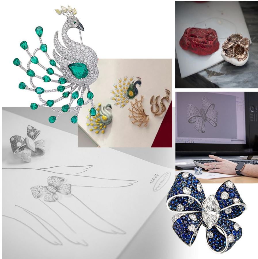
PICCHIOTTI Masterpieces Peacock Brooch , molds and design sketches for peacock brooch, wax mold and rough cast piece, CAD drawing on the computer, PICCHIOTTI Sapphire and Marquise Diamond Fiocco Bow ring , hand drawn design sketch of the Fiocco ring
